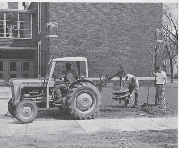
Landscaping —A posthole digger saves many hours with trees and shrubs—both at the nursery and on landscape projects. Helps, too, with signs, swing sets, etc.
