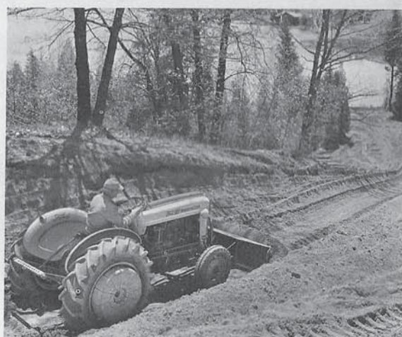
Blade work —Both front and rear blades are available for grading, leveling and backfilling . . . easy maintenance of paths and roads in recreation areas.
